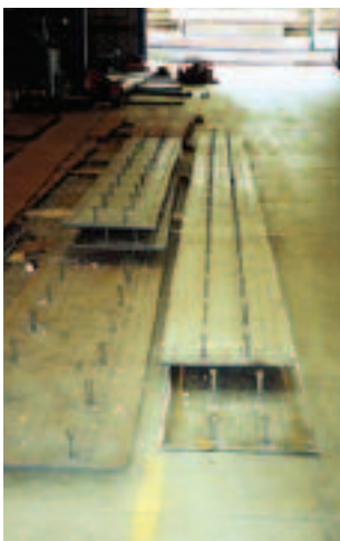
Bisplate 80 plates, with shear studs, prior to forming into box sections.
