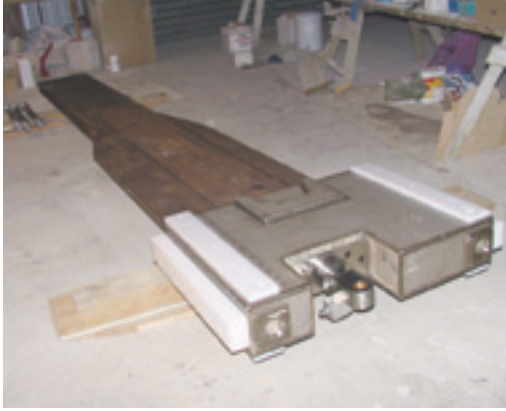
The high strength and narrow profile of BISPLATE are employed with great success in the fabricated box-section keels of the Bakewell-White designed boats.
